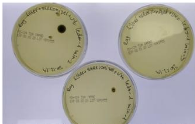
Figure 13: incubation results of the Ray filter+ Air-Reviver+ UVc LEDs plates on December 31 st , 2019
